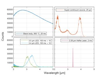
Raw data (no smoothing, post-processing, or pixel binning) showing the emission spectra of four different infrared light source: (top left) 800 °C blackbody, (top right) mid-infrared supercontinuum light source, (bottom left) two different LEDs, (bottom right) He-Ne laser. The legends show the exposure time used to capture the data.
