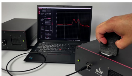
Sample 1. Reflection measurements of a black foam.
